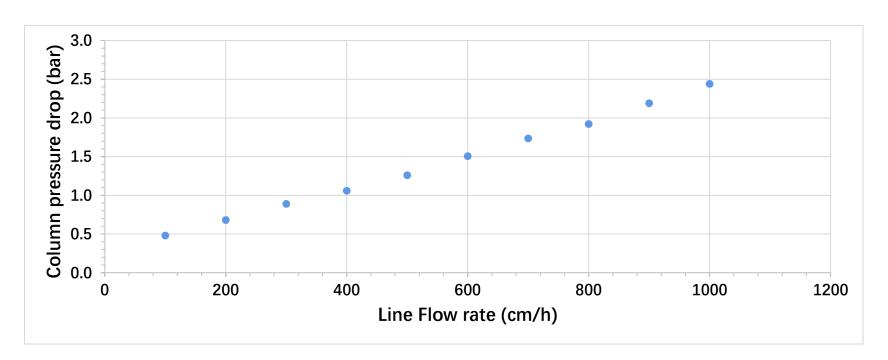
Column pressure drop is around 2.0 bar at 1000 cm/h linear flow rate.
